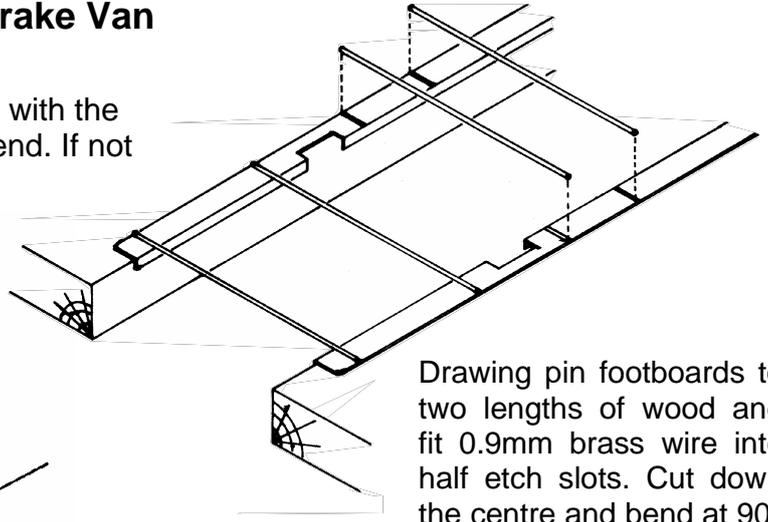
Drawing pin footboards to two lengths of wood and fit 0.9mm brass wire into half etch slots. Cut down the centre and bend at 90° to form footboard supports.
