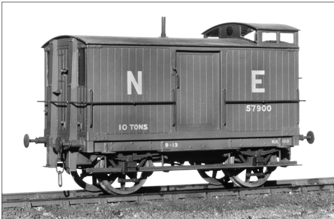
**Prototype.** The diagram V1 brake vans were built by the NER about 1890 -1898. They were a development of similar outside framed vans of much earlier origins and can be thought of as the first standard NER brake van design. They worked in traffic into LNER days and some vans were very long lived with four making it into preservation. A fully restored example is at Beamish Museum.
